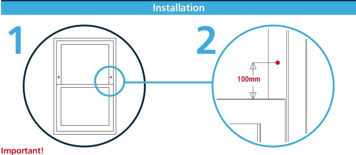
Close and lock sash before starting installation.
