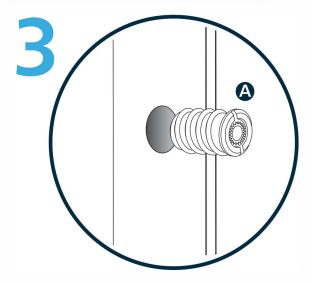
De-activate Push Ventlock™ (A) by pushing the centre button in and turning clockwise.
