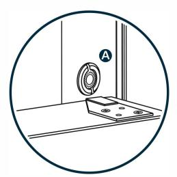
De-activate Push Ventlock™ (A) by pushing the centre button in and turning clockwise.
