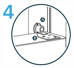
Activate Push Ventlock<sup>™</sup> (A) by pushing the centre button in and turning counter-clockwise. Lower the sash and install the Strike Plate (B).
