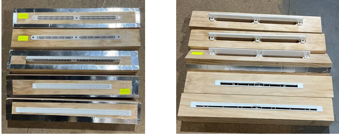
Figure 3 Five samples of trickle ventilator products tested
