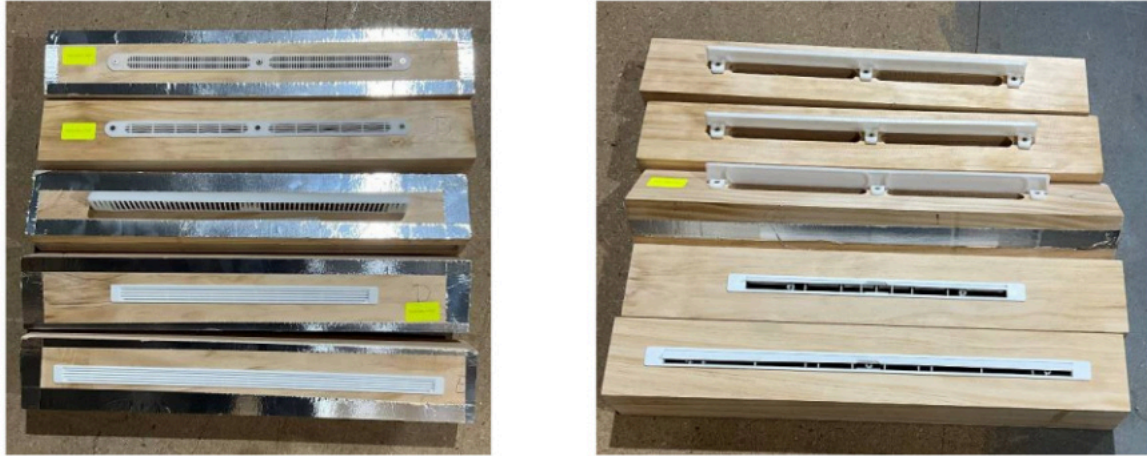
Figure 3 Five samples of trickle ventilator products tested
