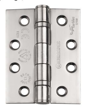
Grade 13 Ball Bearing Hinge (Max Load 120kg) in 2 sizes and 3 Finishes, also Radius version available. Ball bearing hinges have always been very popular for their smooth operation, durability, long lasting design and ability to carry heavier loads than washered hinges. They carry a CE mark and are Certifire tested. BS EN 1935 rated.
