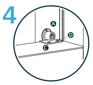
Activate Minilock **(A)** using the Key **(B)** provided. and lower the sash. Install the Strike Plate **(C)** where Minilock **(A)** meets the meeting rail using the Screws **(D)** provided.
