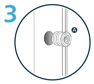
De-activate Minilock **(A)** using the Key **(B)** provided. Screw the Minilock **(A)** into the holes on both sides of the top sash.
