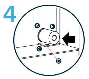
Attach Barrel Unit **(E)** into Insert Unit **(A)** using the Key **(B)** provided and lower the sash. Install the Strike Plate **(C)** where the Barrel Unit **(E)** meets the meeting rail using the Screws **(D)** provided.
