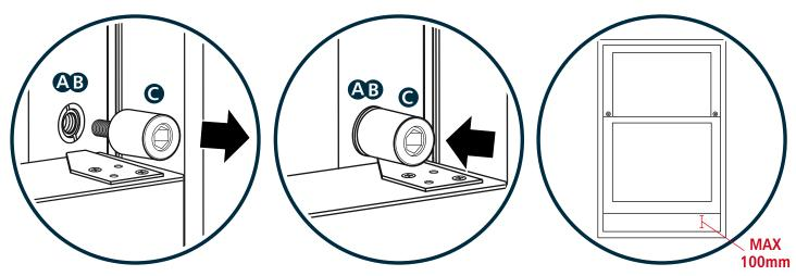
De-activate UniStop by removing the Barrel Unit **(C)** from the Insert **(A/B)** using the key provided **(D)**. Activate UniStop by attaching Barrel Unit **(C)** into the Insert **(A/B)** using the key **(D)** provided.
