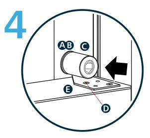
Attach Barrel Unit **(C)** into the Insert **(A/B)** using the Key **(D)** provided and lower the sash. Install the Strike Plate **(E)** where the Barrel Unit **(C)** meets the meeting rail using the Screws **(F)** provided.
