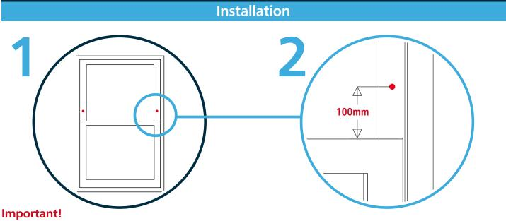
Close and lock sash before starting installation.
