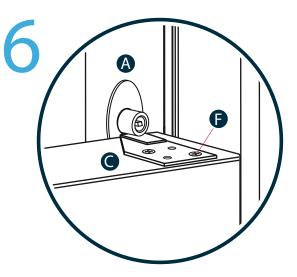
Lower the sash and install the Strike Plate (C) where Locking Ventlock (A) meets the meeting rail using the Screws (F) provided.
