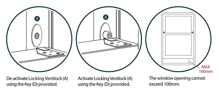
Clean the Locking Ventlock with a damp cloth. On a regular basis, ensure the device operates correctly. Window opening control device installation is now complete.
