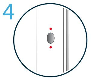
Drill two 3mm diameter holes 15mm deep into the top sash as shown above.
