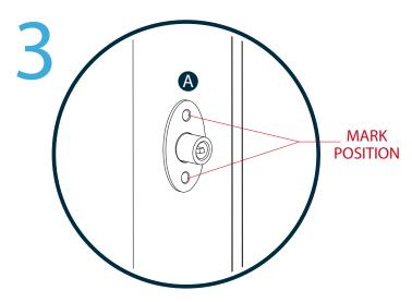
Insert the Locking Ventlock (A) into the hole and align in a vertical position. Mark the sash through the two fixing holes.
