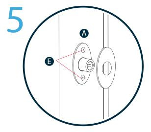
Install the Locking Ventlock (A) onto the top sash using the Rivets (E) provided. Attach the appropriate Face Plate (B) onto the Locking Ventlock (A).
