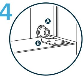
Activate Push Ventlock<sup>™</sup> (A) by pushing the centre button in and turning counter-clockwise. Lower the sash and install the Strike Plate (B).
