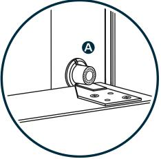
Activate Push Ventlock<sup>™</sup> (A) by pushing the centre button in and turning counter-clockwise.
