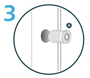
De-activate Push Ventlock<sup>™</sup> (A) by pushing the centre button in and turning clockwise.
