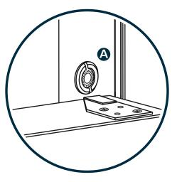
De-activate Push Ventlock<sup>™</sup> (A) by pushing the centre button in and turning clockwise.
