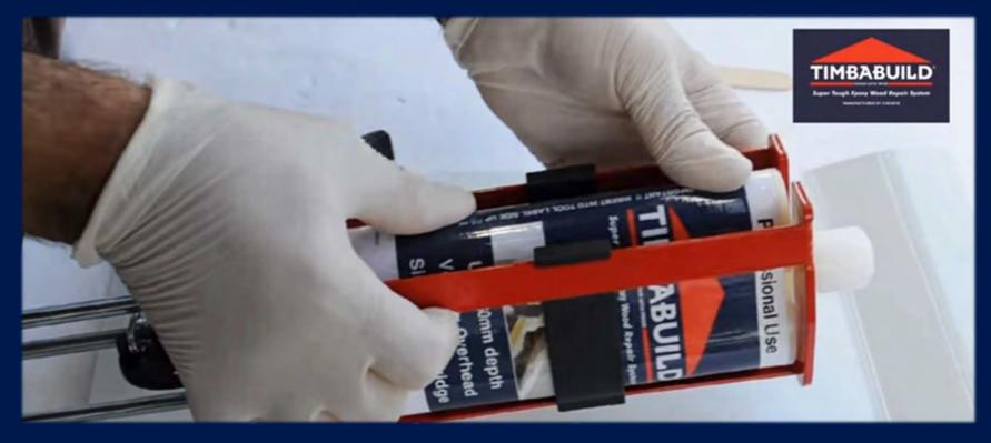
Insert either EHB60 or ERC10 cartridge into the dual cartridge extrusion toolwith the labelled side facing upwards
