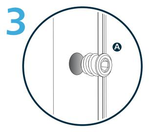
Using a 6mm Allen key, screw the Insert Unit (A) into the holes on both sides of the top sash.
