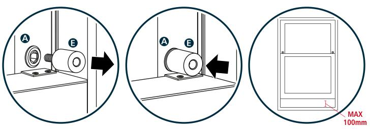
De-activate MigStop by removing the Barrel Unit **(E)** from Insert Unit **(A)** using the key provided **(B)**.
