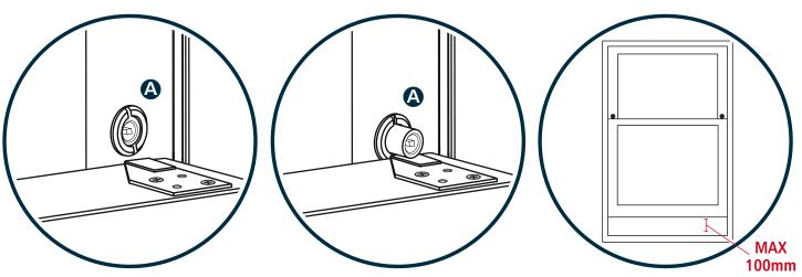
De-activate Locking Ventlock **(A)** using the Key **(C)** provided.
