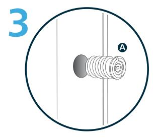
De-activate Locking Ventlock **(A)** using the Key **(C)** provided. Screw the Locking Ventlock **(A)** into the hole using a large flat bladed screwdriver.
