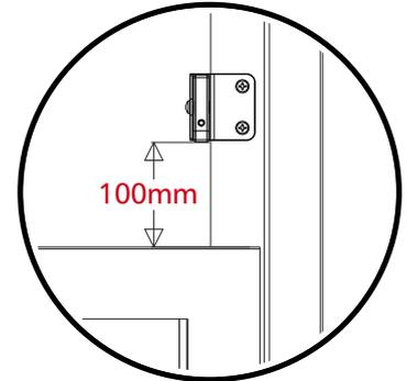
Devices are supplied in pairs and both must be fitted to ensure window is safely secured. One device is fitted to each side of the top sash.
