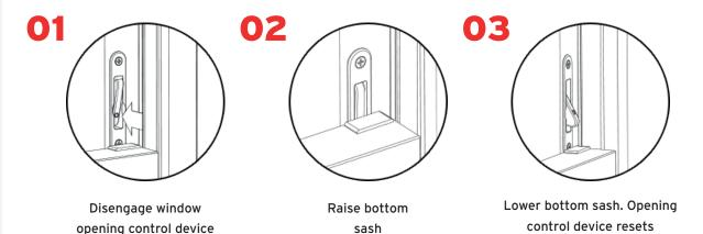
To manually re-engage window opening control device
