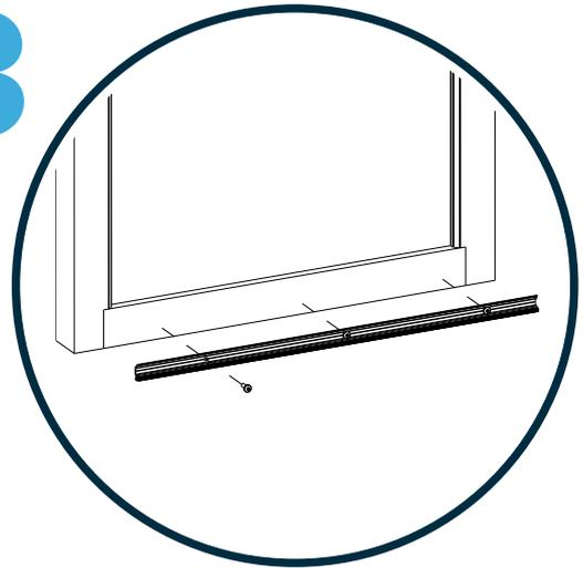
Attach Meeting Rail Interlock (A) onto the first sash using self drilling screws.
