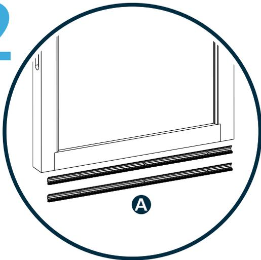
Measure the distance between the parting beads on the window and cut two lengths of Meeting Rail Interlock (A) to fit comfortably without touching the parting beads.
