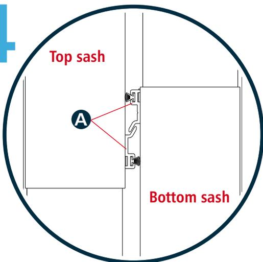
Position and attach the second Meeting Rail Interlock (A) onto the second sash so that the two meeting rails interlock when the window is closed.
